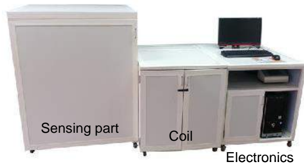
Fig. 2.3. Magnetic immunoassay analyzer XacPro-S is consisted of three modules: sensing part, coils, and electronics.
